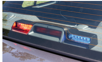
TLNCV5** mounted around 3rd brake light.
