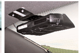
TLN2 with TLNBKT5 mounting bracket shown mounted on headliner over rear deck.
