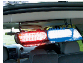
Bracket mounted on interior roof over tailgate.
